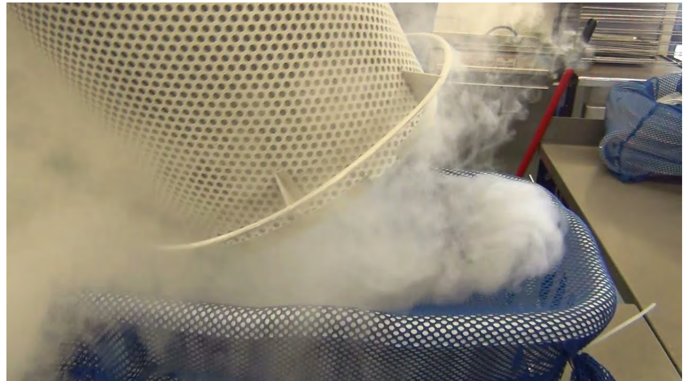
Cryogenic deflashing can be used to remove flash from batches of smaller parts. ( Nitrofreeze )
