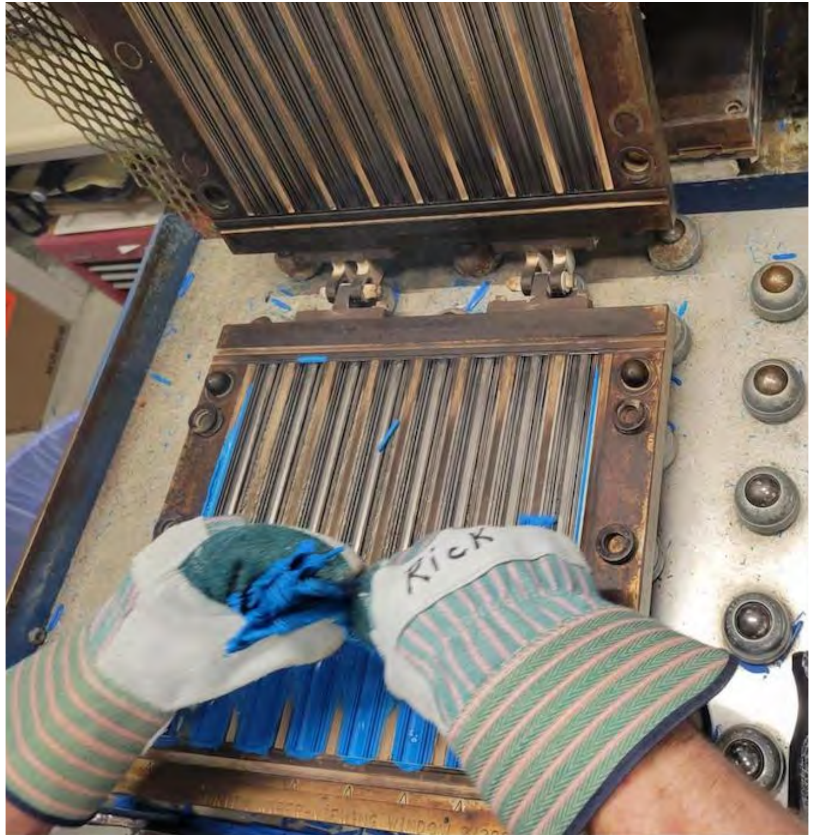
Compression molds are relatively simple but can be used with various materials. (SSP)
